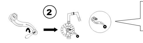
Affix the pump handle onto the crank & connect the crank to the crankshaft on the pump body. Secure the connection using the bolt provided. Make sure that the bolt fits onto the depression in the crankshaft
