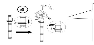
Choose the bung adapter that best fits your drum. Each pack comes with two adapters, which have slight difference in the threads to suit different drums (metal & plastic). Slide the selected 2" bung onto the tube from the top end & tighten the suction tube onto the inlet on the main pump body. Use a thread sealant to connect the suction tube parts for a totally leak-proof connection.
