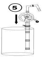
Once the bottom of the pump touches the base of the drum, securely fasten the bung onto the drum. Now very lightly tighten the bung onto the suction tube
