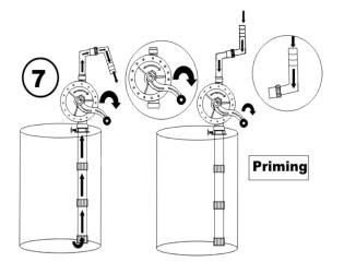
Take an empty container & place it below the discharge spout. Start rotating pump handle. Within a maximum of 7 rotations, pump will be primed & will start dispensing fluid. In a rare case, where the pump does not get primed reverse the outlet discharge spout on the pump & pour about 30 ml of any oil into the outlet & pump the handle for about 7 rotations.
